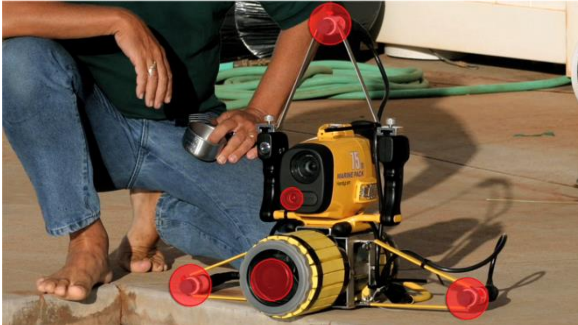
Figure 2. Photo of the “pre-runner” system – consisting of a Sony underwater housing with camera, three hydrophones and the computer section with a PC104 system.
